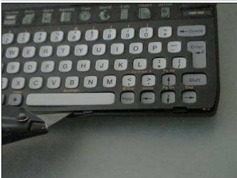
3. Using a blunt knife, release the two centre tabs on the bottom edge of the key surround.
