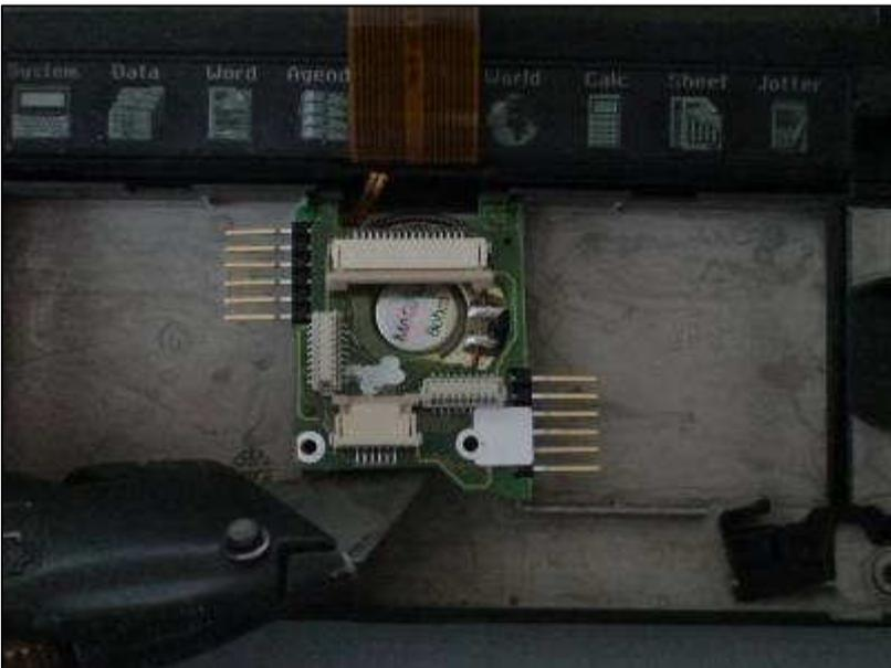
11. With a blunt knife, lift the seaker PCB at the front and pull forward to release the rear tabs. CAUTION: You may need to release the flexi and rubber elastomeric strip.
