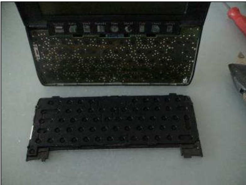
5. In order to remove the keys and membrane you have to ensure that the key caps do not all fall off. To do this, put the key surround back over the keys and 'flip' the surround and keys over to leave the membrane on top of the surround as shown. Put the assembly aside for later.
