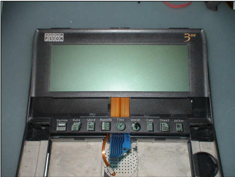
28. Refit the screen by sliding the screen flexi and backlight flexi under the blue icon bar flexi. Ensure the bottom of the screen is in the screen casing and gently slide down ensuring the flexi's do not get snagged. Clip the tabs at the top of the screen back under frame. Now replace the two screws on the outer of the screen casing to secure the screen.
