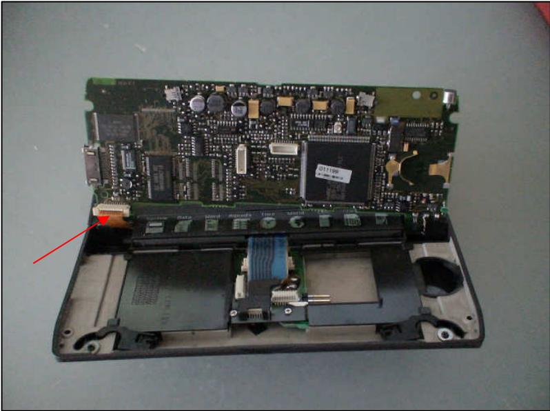
7. Lift the motherboard to reveal the battery flexi as shown in the diagram. Remove the flexi from the ZIF socket by lifting the two tabs on the side away from the motherboard. Remove the motherboard and put it aside for later.
