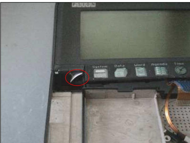
15. Remove the rear cover by gently bending the flexi as shown to get it through the hole in the main unit.
