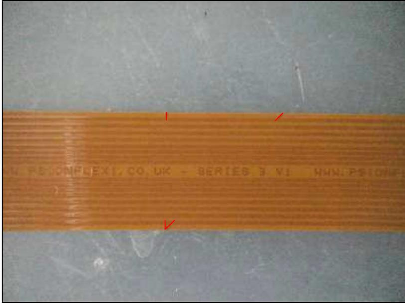
24. With the text uppermost and the folded end to the right, locate the centre folding alignment marks shown highlighted.
