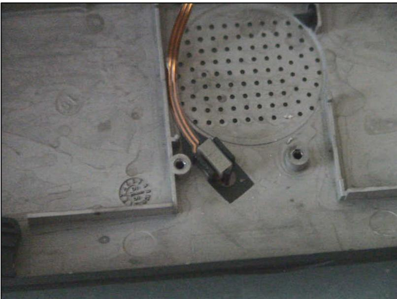
29. Replace the backlight flexi onto the two pins in the base and place the elastomeric block back between the two pins.
