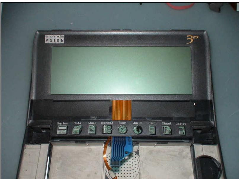
18. Now remove the screen by gently lifting the top forwards and sliding the screen upwards. Be very careful that the two flexi's do not get tangled/trapped.
