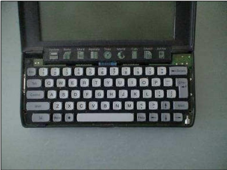
4. Lift the front of the key surround so that the rear tabs are released. Remove the key surround to leave the machine looking like the picture.
