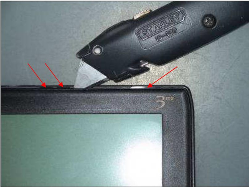
16. Using a blunt knife, pop the tabs on the screen bezel out from the screen frame. There are two large ones on either side and two in the centre.
