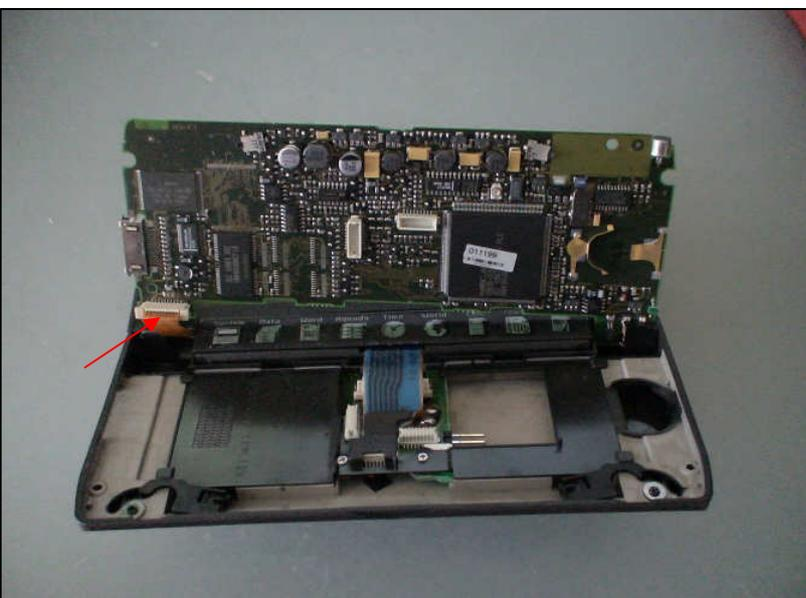
33. Connect the power flexi (on the left of the icon bar) to the motherboard ZIF connector, ensuring that the two tabs are pushed away from the flexi fully.
