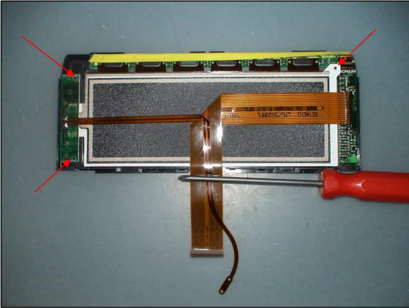
19. Once the screen has been removed, turn it over and note that the longer thinner backlight flexi is on top of the screen flexi (the thicker one). Also note that the backlight is located on the 3 pins shown.
