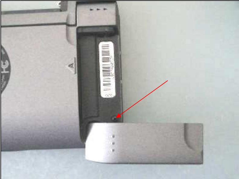
1. Remove the screw under the left hand memory card cover as shown/
